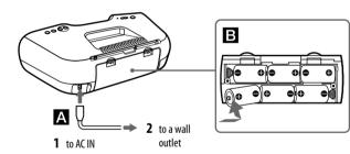
Connect the AC power cord A or insert six R20 (size D) batteries (not supplied) into the battery compartment B.
